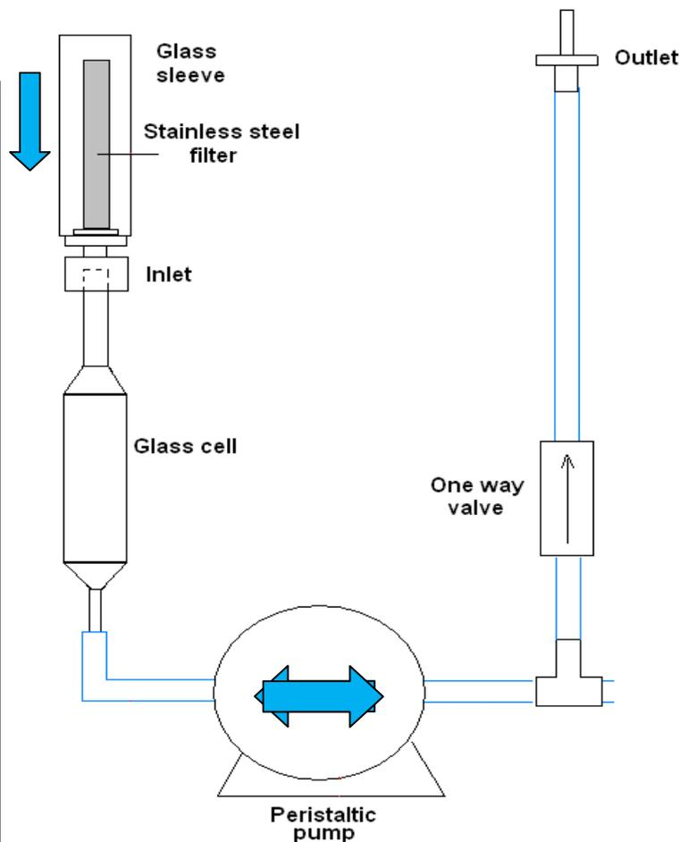
**Capable of sampling both dissolved and particulate fraction.**
