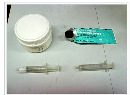
Krytox fluoroether-based grease (left) is often used in laboratories, including in high-vacuum applications,
